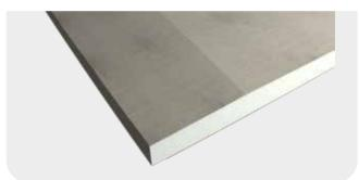
Gyproc Protect F<sup>®</sup> is a fire-resistant plasterboard with significantly better fire resistance properties than ordinary plasterboard. The desired fire class can therefore be achieved using fewer board layers compared to standard plaster. The board consists of a core made from high-density fibreglass-reinforced plaster with dimension-stabilising mineral additives and a cardboard surface layer. The board thickness is 15 mm. ISOVER PLUS+
