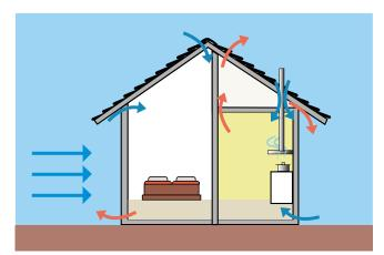
Illustration 6. Permeable house with poor control of airflow.
