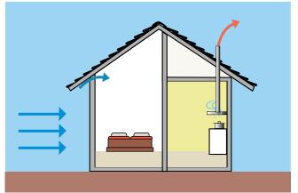
Illustration 7. Non-permeable house with control of airflow.
