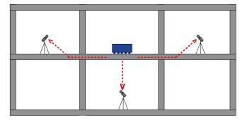
The illustration shows how footstep impact sounds from an impact device can spread in a building. If a low footstep impact sound level is measured in a room, the joists have high footstep impact sound insulation. The BBR requirement concerning footstep impact sound levels is a field value designated L'<sub>nTw</sub>.
