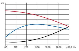
The black line shows the sound level at various frequencies from the chirping of birds, the blue line shows a voice and the red shows an idling lorry.
