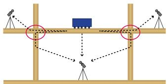
Illustration 2 shows a field measurement. The field value is designated  $L'_{nT,w}$  and is affected by flank transmissions via the framework in addition to the footstep impact sound insulation in the joists. The panel points (highlighted in red in illustration 2) must be executed correctly to prevent footstep impact sound from spreading into adjacent rooms.
