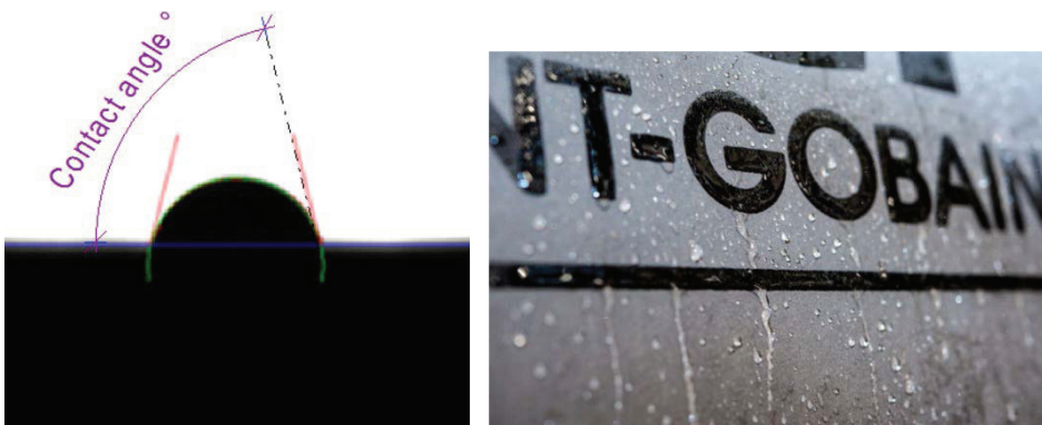
Fig. 1 The contact angle of a drop with respect to the surface.
