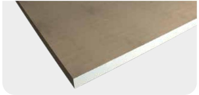
Gyproc floor plasterboard allows for “dry” solutions with good airborne and footstep impact sound insulation on top of a subfloor. The board consists of a core made from high-density fibreglass-reinforced plaster and a cardboard surface layer. The board thickness is 13 mm. The boards can be supplied in accordance with Saint-Gobain’s Construction optimization concept.
