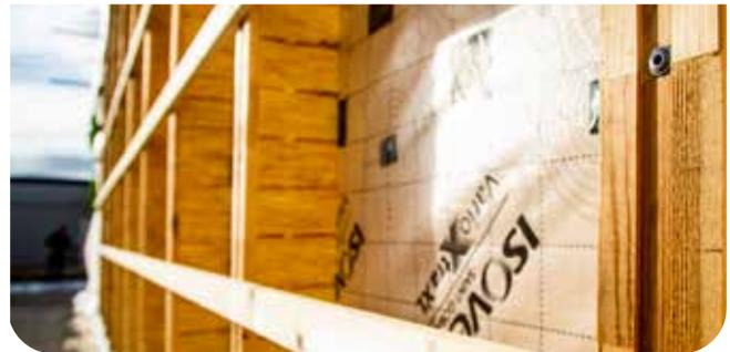
ISOVER Vario<sup>®</sup> Xtra is a non-woven reinforced variable vapour retarder. The product is used for air sealing and moisture protection in walls, floors and roofs. Unlike ordinary PE film, it adapts to the relative humidity (RH) of the retarder:
