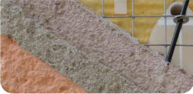
Serporoc Premium 32 Façade system is a thick mineral stucco system on glass wool plaster carriers with insulation thicknesses of 30-120 mm. With its strong stucco structure, the Serporoc system is highly suitable for environments where the façades are exposed to great stress.
