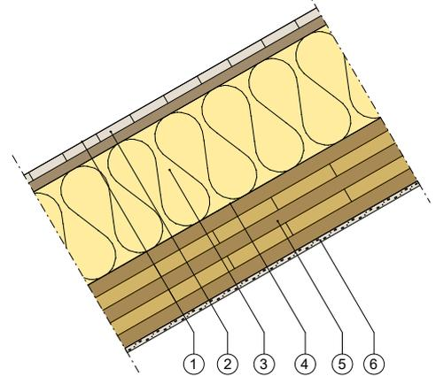
1. 2 mm Roof covering/roofing felt
