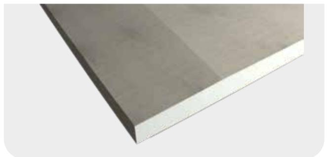
Gyproc Protect F® is a fire-resistant plasterboard with significantly better fire resistance properties than ordinary plasterboard. The desired fire class can therefore be achieved using fewer board layers compared to standard plaster. The board consists of a core made from high-density fibreglass-reinforced plaster with dimension-stabilising mineral additives and a cardboard surface layer. The board thickness is 15 mm.
