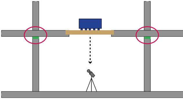
Illustration 1 shows a footstep impact sound measurement in joists at a laboratory. The framework in the laboratory has been “soundproofed” so that no sound can pass to the receiving room via the framework. The laboratory value for the joist is designated  $L_{n,w}$  and shows only how much sound passes through the joists.
