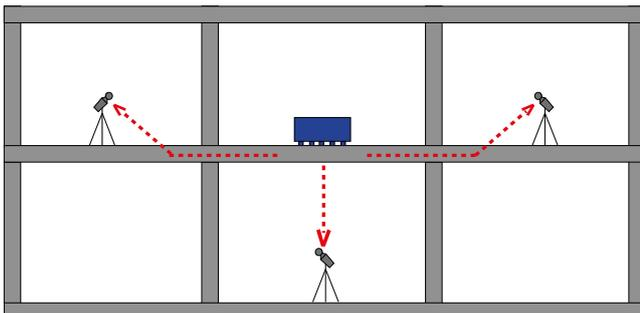
The illustration shows how footstep impact sounds from an impact device can spread in a building. If a low footstep impact sound level is measured in a room, the joists have high footstep impact sound insulation. The BBR requirement concerning footstep impact sound levels is a field value designated  $L'_{nT,w}$ .
